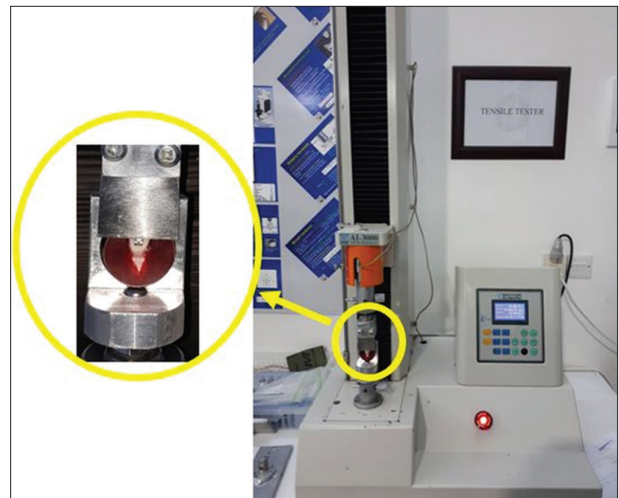
Figure 2: Universal testing machine GOTECH (shear bond strength)
