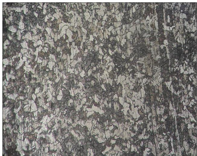
**Figure 2: Microstructure of as received low-carbon steel AISI 1018(x600)**
