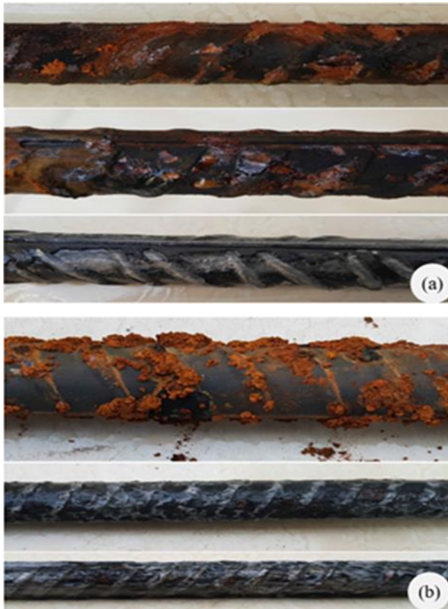
Fig.6. corrosion of the specimens after 5 years of exposure (a) immersed in salty water (b) detergent solution.
