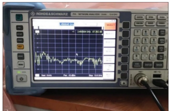
Figure 9: The vector network analyzer Rohde and Schwarz® ZVL13 with a frequency range of 9 kHz ~ 13.6 GHz
